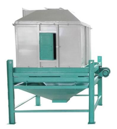
The cooling and screening process is the process that can reduce finished pellets' temperature from about  $80~^{\circ}\text{C}$  to room temperature and to reduce the moisture from about 15% to 12%. To achieve a better storage, this process is in need. Using our biomass cooler, the finished pellets' recherche will be less 3-5  $^{\circ}\text{C}$  higher than the room temperature.
